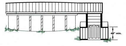
The latch must be placed on the inside of this gate.
